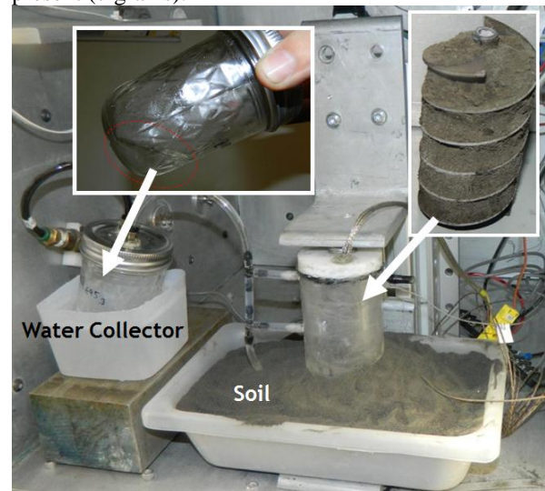
Figure 4. MISME water extraction system being tested in Mars chamber.
